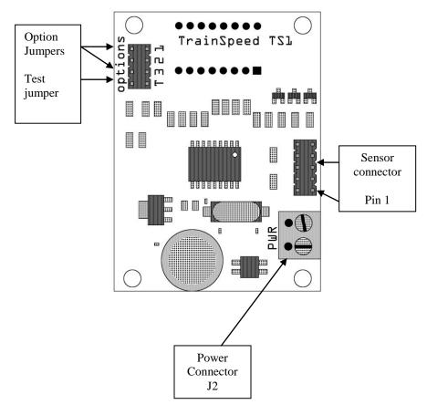
6v-18v AC or DC Input polarity does not matter
