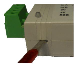
Identify the location for the jumper link near the DCC input connector, see below.
